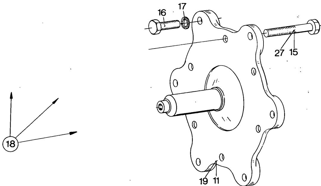
SLIP CLUTCH AND OVER-RUNNING CLUTCH
